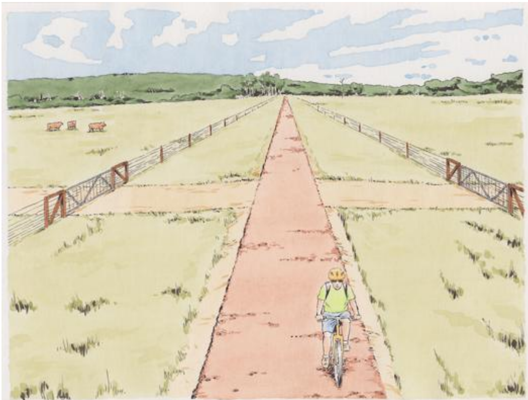
Above: Stock Crossing Type A: crossing open 24/7 for stock and machinery. Below: Stock Crossing Type B: Trail open 24/7. Gates in side fences.
